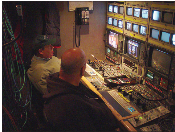
Figure 6.28 The video operators are charged with maintaining the correct video levels and ensuring that all the cameras have the same "look." The director often only notices video operators when it is obvious that they are doing a good job under adverse conditions, or if they are doing a poor job.
