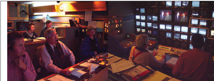
Figure 6.18 A couple of shots of the "bridge" of the production truck, the production compartment. The TD, director and producer sit in the front row in most trucks. The producer generally writes the story, which the director tells through the TD, A1 and the graphics people. Additional people in the production compartment usually include associate directors and producers, who are most often there to help with the flow of graphics and replays. Steve notes that the "chemistry" among the crew, and especially in this compartment, can determine if the shoot is a smooth, good one, or if this outing will be a struggle.
